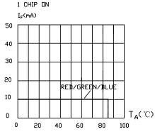
MAXIMUM FORWARD DC CURRENT VS. AMBIENT TEMPERATURE
